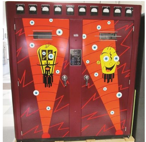
Not all of Moersdorf's transmitters are kept "stock," as exemplified by this now one-of-a-kind Gates BC-1F 1 kW model from the early 1950s. (Moersdorf has another with Parker Gates' factory paint job.)
