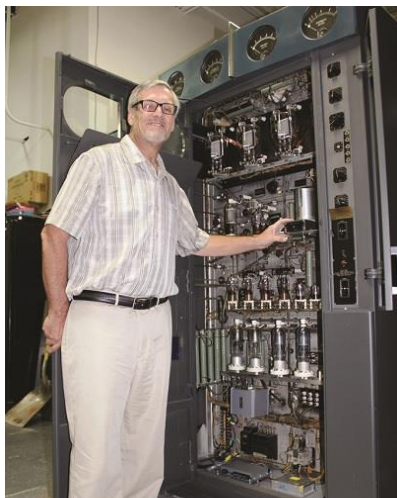
Gerry Moersdorf shows off the oldest item in his large collection of broadcast transmitters. The Western Electric 443A1 1 kW Doherty dates to the 1940s. Moersdorf notes that it tunes between 550 kHz and 2,750 kHz, allowing it to be used in the old police
