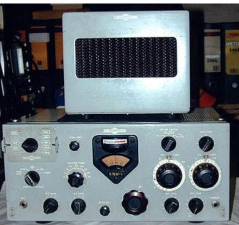
A Collins KWM-1, an early Amateur Radio transceiver that featured SSB voice capability
