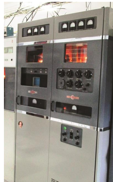
Moersdorf's collection contains only one non-broadcast transmitter, this Collins AN/FRT-24 1 kW base station transmitter built for the U.S. Navy. It tunes 2–30 MHz and was constructed in the mid-1960s.
