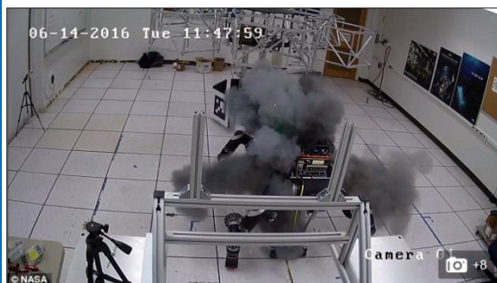
The machine begins to smoke as its batteries begin to combust
