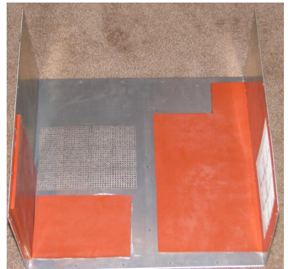
Modified AL-1500 Cover with rubber glued in place for sound dampening.
