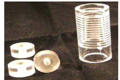
The coil form has a thread cut into it to guide the wire winding. This will make it easier to wind the coil.
