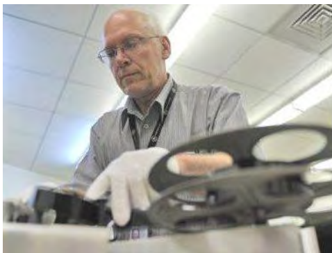
Engineer Russell DeMuth sets up a film in the machine he built to read the optical audio film that was over 80 years old at the Schenectady Museum & Suits-Bueche Planetarium in Schenectady. (Skip Dickstein/Times Union)
