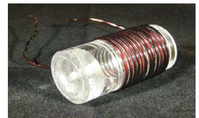
The 10 Meter coil has 12 turns of 16 Ga. wire at 11 TPI.
