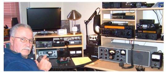
Collins KWM-2 with rejection tuning mod. The KWM-2 is connected to a Drake W-4 watt meter.
