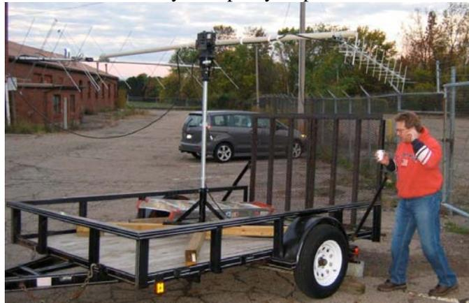
assembled it and mounted it the same base that he used for his forty meter inverted vee at Field Day and then trailered it to the club site. Fortunately it looked as though he had only put a slight bend in two of the two meter beam elements as a result of some "harmful interference" on the way up.
